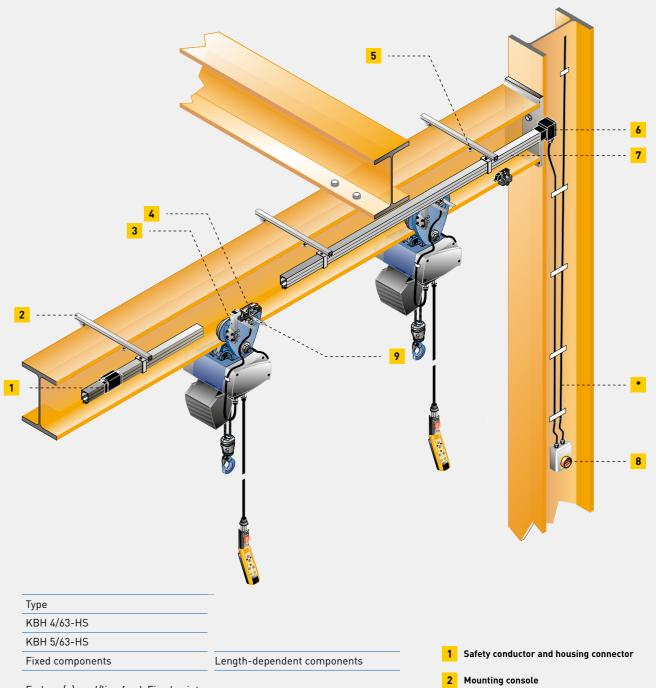
End cap(s), end/line feed, Fixed point suspension, Collector with 2 m connection cable, collector fork and mains switch
