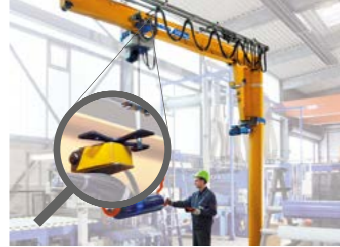
Limit switch for cross travel (Fig. 8)
